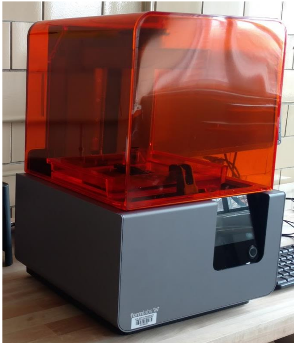
Form 2, Formlabs Desktop 3D Printer
