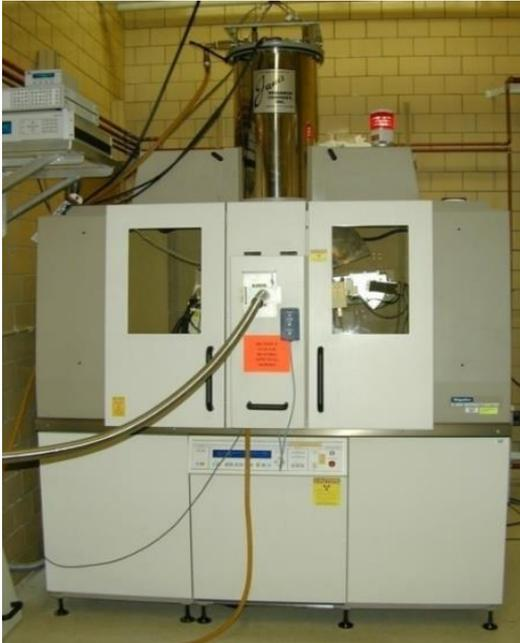
**Rigaku TTRAX** rotating-anode powder diffractometer with a custom-built cryostat & superconducting magnet
